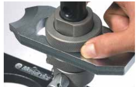
Adjusting the gear according to the size of the spring coil
