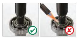
Heating up bearing will cause heat to transfer and damage tool  $% \left\{ \left( 1\right) \right\} =\left\{ \left($
