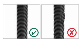
Frequently lubricate and inspect forcing screw for damage  $\,$
