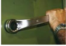
Where extra leverage on tough fasteners is required
